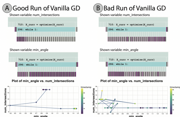
Fig. 9. Using Anteater to compare two runs of the Vanilla gradient descent that should maximize the minimum crossing angle while minimizing edge crossings. In (A) we see that the number of intersections rapidly decreases while the minimum angle increases. In contrast, in (B) we see that the number of intersections is increasing throughout the descent while the minimum angle decreases.
